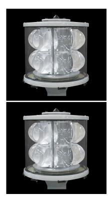
Rotating beacon, 25NM @ 0.74T. The VRB-25 LED is a high intensity rotating beacon suitable for ranges up to 25 nautical miles. Being an LED beacon, it is extremely energy efficient and can be monitored digitally. It is an ideal replacement for beacons with Fresnel lenses in historic lighthouses, or locations requiring intensities greater than what can be achieved with typical stationary beacons.
