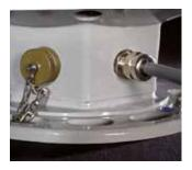
Additional cable entry Equipped as standard with two cable entries. If the secondary entry is needed e.g. for a solar module standard M20 cable gland can be fitted.
