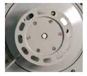
Installation The bottom plate of the LED 350 supports installation on structure using 3 x M12 bolts or 4 x M12 bolts on a 200 mm diameter.
