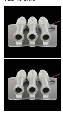
21 - 25NM by night @ 0.74T, 3.9 - 6.2NM by day @ 0.74T. The VLS-46 Ultra is ideal for harbours with narrow or difficult approaches. The modular design allows up to seven projectors to be placed side by side. This can be used to create unique sector angles, flash patterns and intensities. The VLS-46 Ultra has been designed to take advantage of the latest LED technology.
